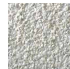
M: Medium [3-5 mm] Thickness: 8.0 ± 0.6 mm
